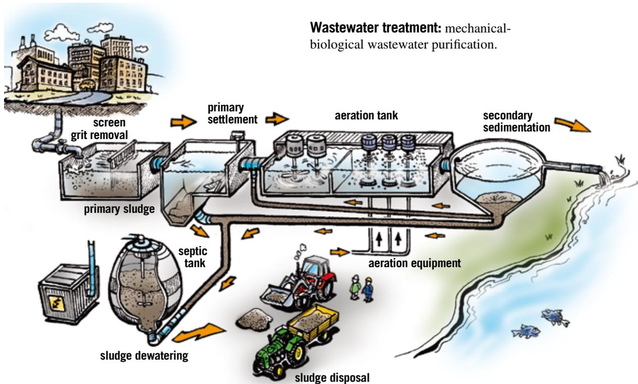
**Wastewater treatment:** mechanical-biological wastewater purification.
