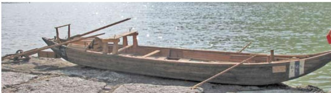
**“Sieberin”:** This type of ship was used for the transport of salt.
